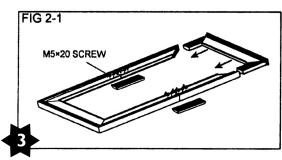
Connect short side last by inserting both corner pieces simultaneously. This will prevent distortion and possible damage to frame.
