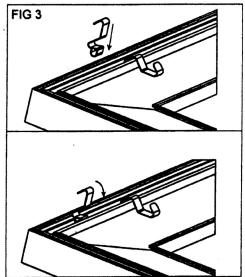
Attach the prepared fabric to the frame, using spring hooks in frame - short edges first.
