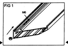
Slide  $4 \times M6$  nuts into the long side slot, and  $1 \times M6$  nut into each short side slot. (**FIG** 1)
