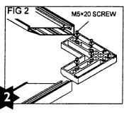
Insert plastic L-shape corner pieces to connect them (FIG 2) NOTE: Refer FIG 2-I
