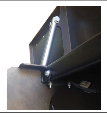
Step 4: Now attach the Mounting Plate & Motor to the Base & Supports.
